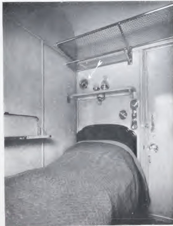
FIG. 1.—Compartment in sleeping car on Railway Carriage showing "Thermo-Reg" Louvres situated above bed-head shelf.
